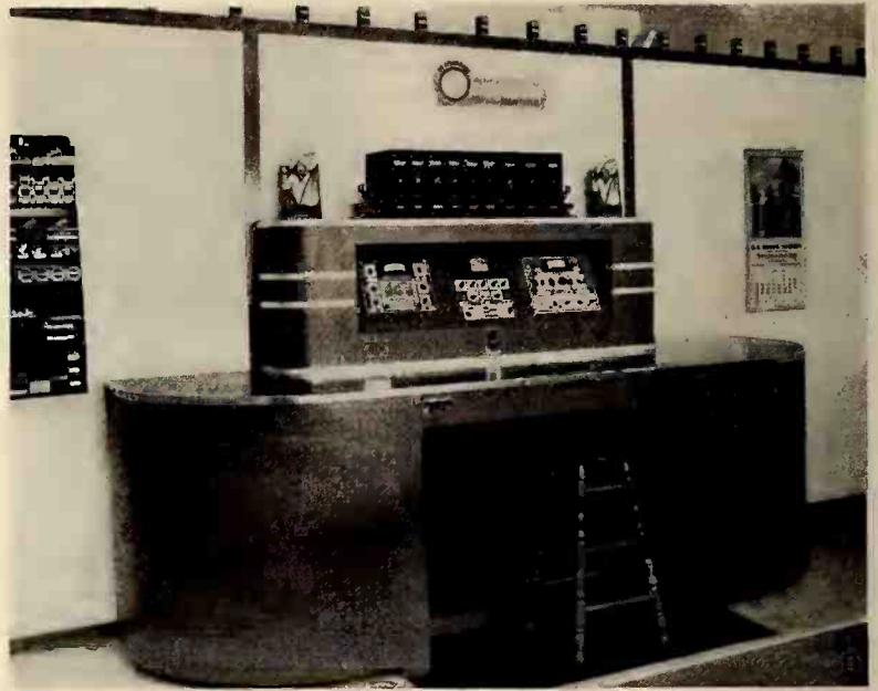
A recent winner in the Sylvania shop modernization contest was Burbank Radio Service, San Jose, Cal. The bench top is of tempered pressed wood. Indirect lighting illuminates the inclined panel.
