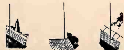
Flat Roof Ridge Pole Parapet
